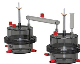
Corrolytics' test kit uses UA technology to better diagnose the cause of corrosion
